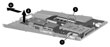
Removing the System Board
